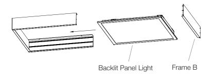
Reattach Frame B to the fixture.
