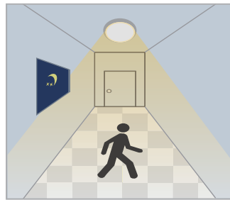
With insufficient ambient brightness, the light dims to 100% when motion detected.
