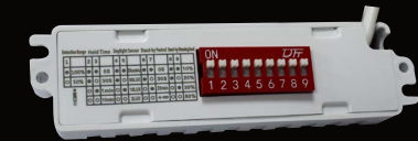
HD016VCR 2 DIP switches on back
